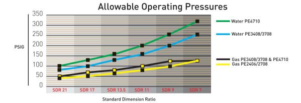
NOTE: Operating Pressure for Conventional Tapping Tees and Conventional Branch Saddles are determined by the material used, the outlet SDR and the governing regulations.
