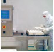
An optimized one hour, four step process: washing, rinsing (two times) and drying is performed for all moulded SYGEF® Plus components.
