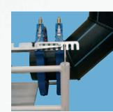
The sliding 3rd clamp provitime saving and a highly fle system for clamping bends tees without additional tool. Just take out the spacer blashift the clamp to the desig position and fix it again with spacer. A double-sided pull mechanism enables a secul heater plate separation from melted pipe ends in all weld positions.
