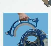
The new tilting upper clamps allow quick and easy pipe securing, alignment and removal of the welded pipe. Whenever necessary, upper clamps may also be quickly removed.
