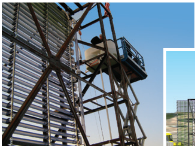
Each BioBlade unit features its own 250-gallon water tank and pump.
