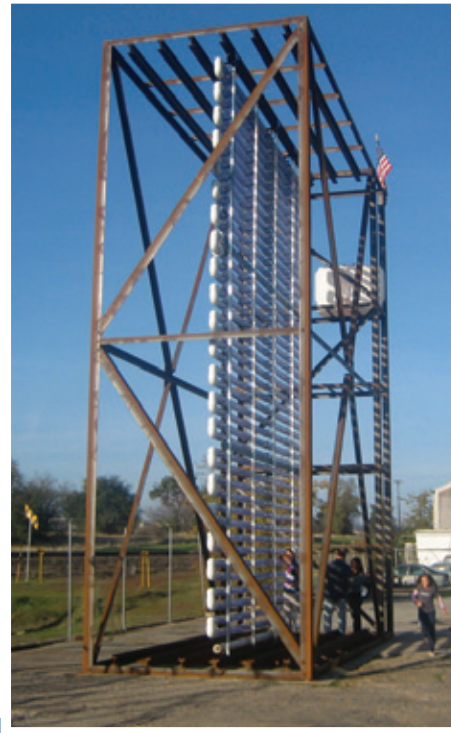
BioBlades are slid into the Photo BioReactor structure in a manner similar to computer server “blades” being slid into a chassis.
